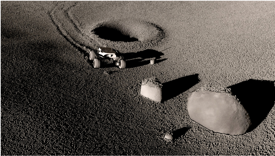
Figure 6.3 – High-fidelity simulation environment with millions of discrete particles used for fine-tuning. This setup provides a more realistic model of wheel–regolith interaction dynamics.
