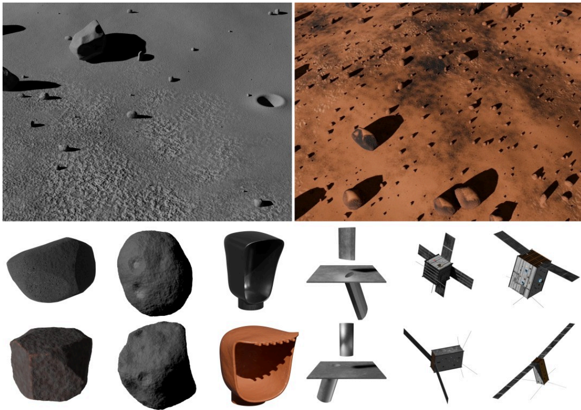
Figure 4.8 – Examples of procedural assets generated by SimForge, including varied terrains, rocks, and structured 3D models like excavation tools, peg-in-hole modules, and spacecraft.
