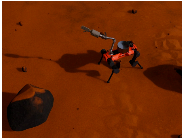
Figure 4.2 – An example of the modular composition of robots in SRB. The framework allows for the combination of any mobile base with any manipulator and any EE to create novel mobile manipulation systems.
