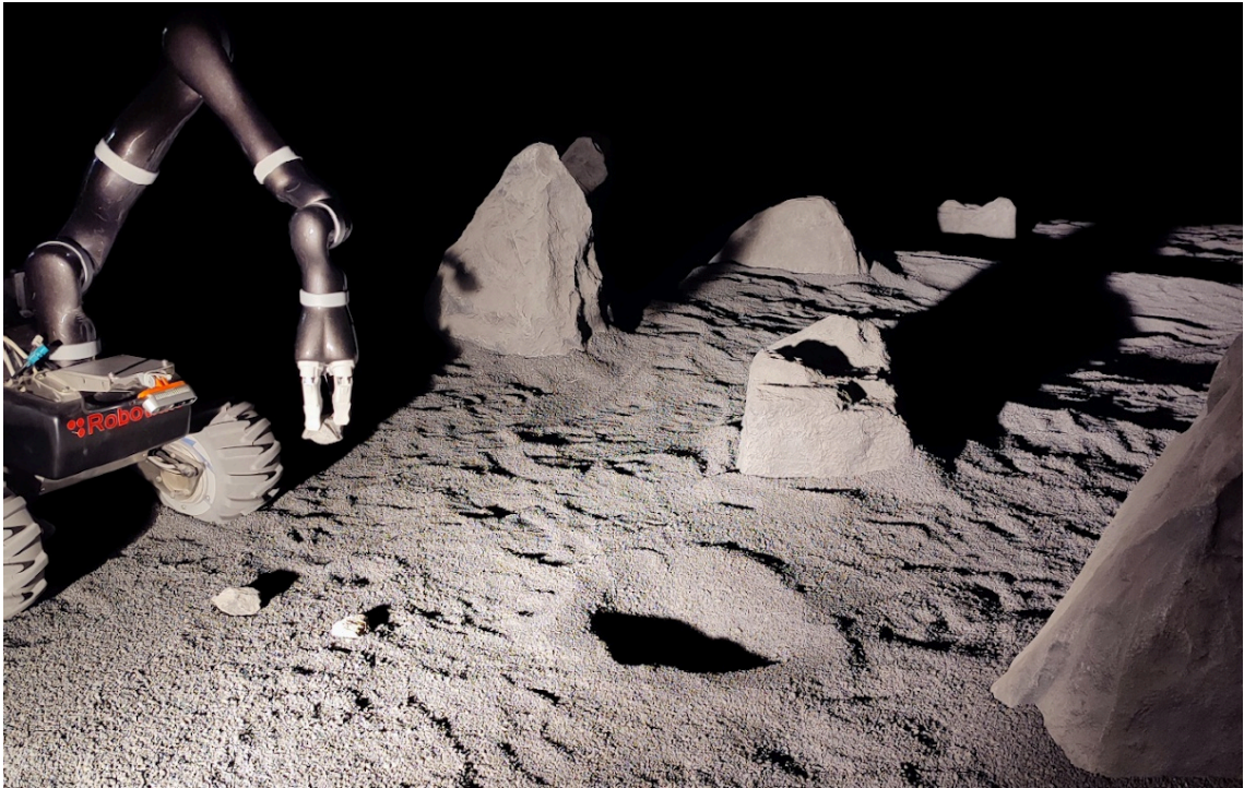
Figure 3.7 – The physical setup for the sim-to-real validation experiments, conducted in the LunaLab facility at the University of Luxembourg. It holds 20 tons of basalt gravel [37].
