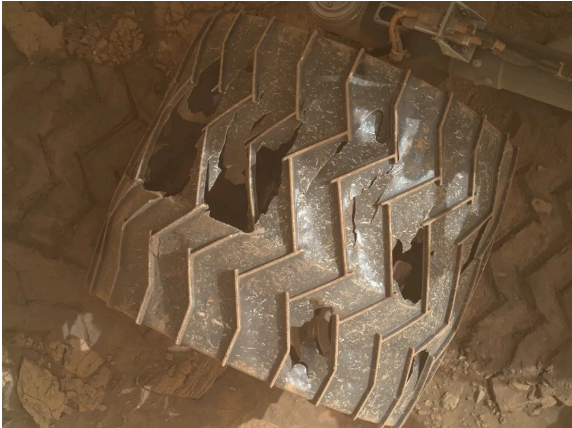
Figure 1.3 – Damage to the wheel of the NASA Curiosity rover on Mars. This image highlights the challenges posed by hazardous planetary terrains, where sharp rocks can cause significant hardware degradation over time [13].
